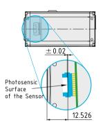
degrees of freedom. The back focal length on each camera is carefully measured and adjusted by our unique "CSAT" procedure. This guarantees an optimum distance between the lens flange and the sensor and ensures outstanding image quality based on compliance with optics standards.
